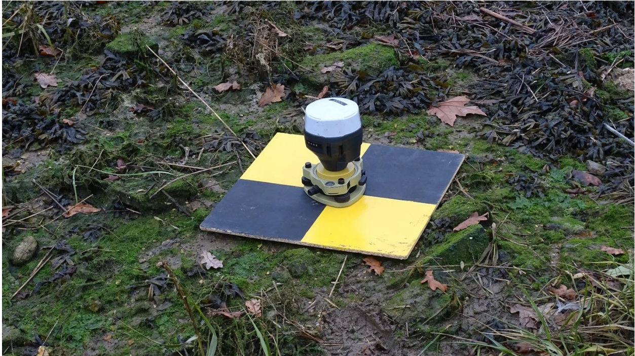
Figure 3.9: GCP positioning (Photo: AQASS, 2021)
