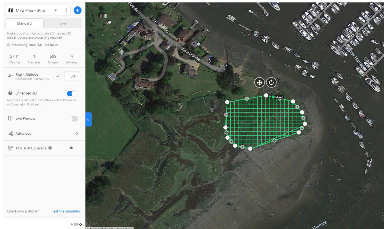
Figure 3.7: Flight plan for surveys (Image: SAND Geophysics, 2021)
